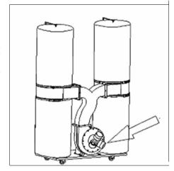
When the dust collector has been fully assembled, a second check should be carried out to ensure that all of the nuts, bolts and bags etc. are fitted correctly and are fully secure. After the re-inspection, you can connect the machine to a power source and have a trial run (see page 15 for operating instructions).
