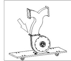
Insert the 2 x gaskets onto the connector and fit the 2 x collectors; ensure that the holes all line up and secure in place with the provided bolts.
