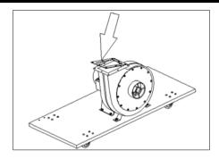
Fit the inlet connector over the gasket ensuring that the holes all line up. Secure in place with the bolts, washers and nuts provided. Fully tighten secure in place.
